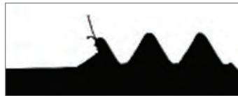
Mounting Post using TECHSPEC® 1X Silver Series Telecentric Lens and Telecentric Backlight Illuminator
