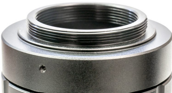
Figure 8: Threaded screw mounts (TFL lens shown above) are machined into a solid piece of metal allowing for vastly stronger clamping force with the camera. This eliminates wobble or sag even with vibration or gravity, regardless of the lens size. TFL is also a published standard.
