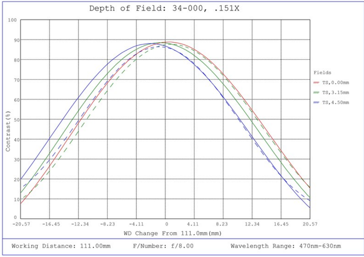
#34-000, 0.151X, 1/1.8" C-Mount TitanTL® Telecentric Lens, Depth of Field Plot, 111mm Working Distance, f8
