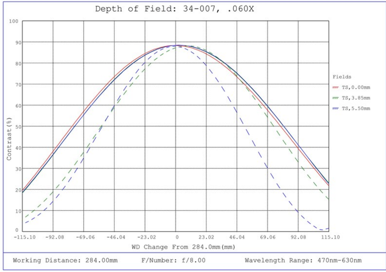
#34-007, 0.060X, 2/3" C-Mount TitanTL® Telecentric Lens, Depth of Field Plot, 284mm Working Distance, f8
