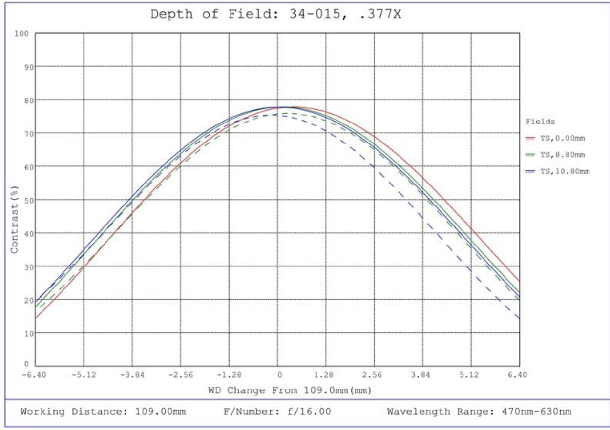
#34-015, 0.377X, 4/3" C-Mount TitanTL® Telecentric Lens, Depth of Field Plot, 109mm Working Distance, f16
