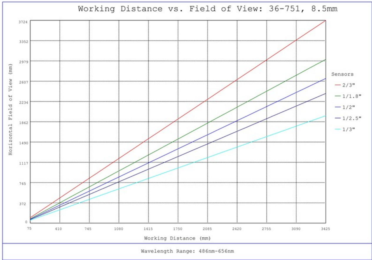
#36-751, 8.5mm f/5.6, 75mm-∞ Primary WD, HRi Series Fixed Focal Length Lens, Working Distance versus Field of View Plot
