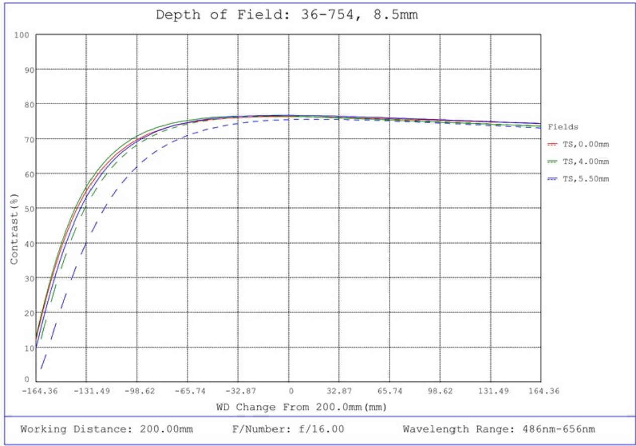
#36-754, 8.5mm f/16, 75mm-∞ Primary WD, HRi Series Fixed Focal Length Lens, Depth of Field Plot, 200mm Working Distance, f16
