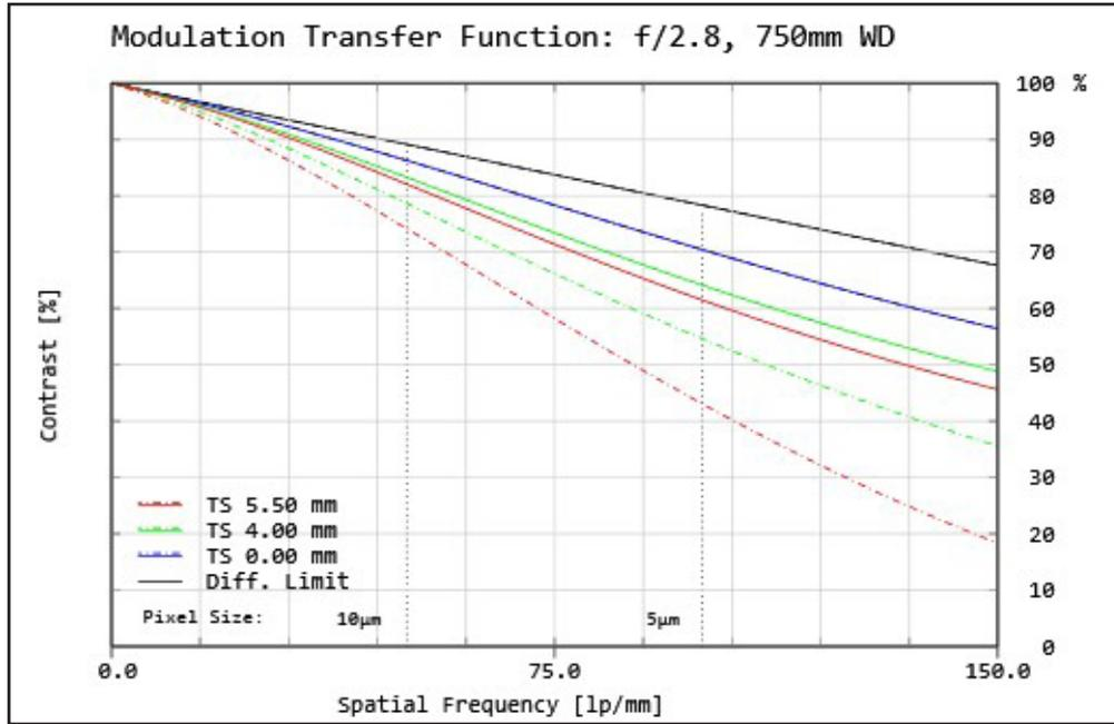
**Figure 7:** Image space polychromatic diffraction FFT Modulation Transfer Function (MTF) for  $\lambda = 486\text{nm}$  to  $656\text{nm}$ . Included are Tangential and Sagittal values for field points on center, at 70% of full field and at the maximum sensor format. Solid black line indicates diffraction limit determined by  $f/\#$ -defined aperture. Frequencies corresponding to the Nyquist resolution limit of pixel sizes are indicated.
