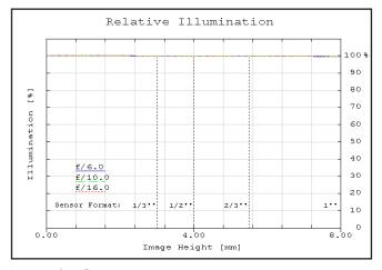
Figure 2: Relative illumination (center to corner)
