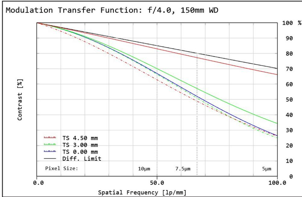
**Figure 9:** Image space polychromatic diffraction FFT Modulation Transfer Function (MTF) for  $\lambda = 486\text{nm}$  to  $656\text{nm}$ . Included are Tangential and Sagittal values for field points on center, at 70% of full field and at the maximum sensor format. Solid black line indicates diffraction limit determined by  $f/\#$ -defined aperture. Frequencies corresponding to the Nyquist resolution limit of pixel sizes are indicated.
