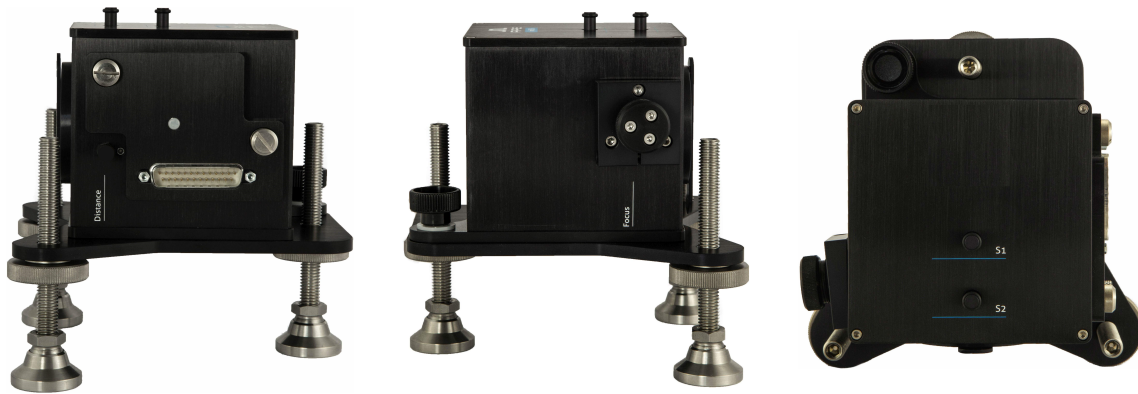
Figure 3.1.: autocorrelator optical head - data cable connection and detector (left), focus position screw (middle), shutter buttons S1, S2 (right)
