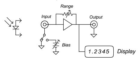
Current input to the unit generates a voltage across the range feedback resistor. This voltage is then measured and displayed in units of amperes. A variable bias voltage may be introduced in series with the detector in use. The output presented is calibrated such that 2.0000V represents the full scale range in use, e.g. 2.0000 V corresponds to 20.000 nA and so on.
