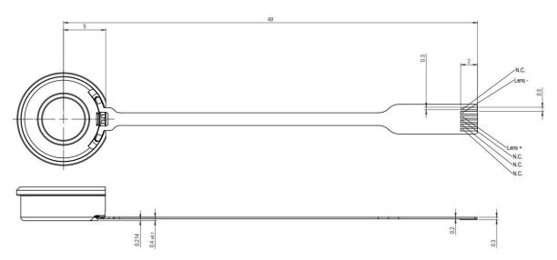
Figure 2: Mechanical drawing of the EL-3-10-XXX-26D-FPC lens
