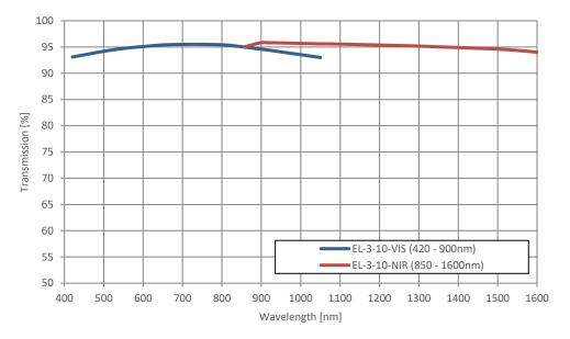
Figure 8: Transmission spectra of EL-3-10 standard VIS and NIR coating
