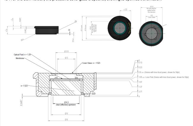
Figure 1: Mechanical drawing of the EL-3-10-XXX-26D-OEM lens
