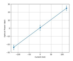
Figure 7: EL-3-10 typical current vs optical power graph
