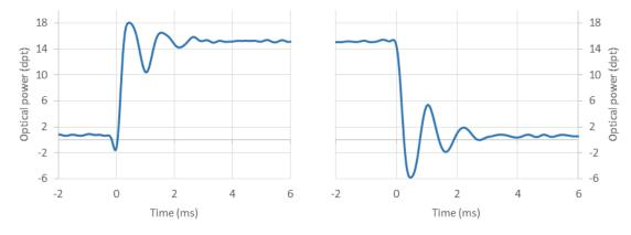
Figure 10: 80% step response of the EL-3-10 lens
