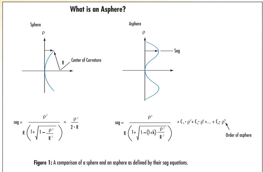
Figure 1. A sphere and an asphere are defined by their sag equations.
