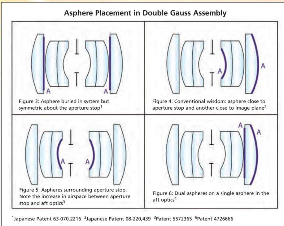
Figures 3-6. Alternative approaches to asphere placement in Double Gauss lens assembly.
