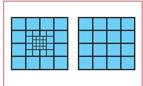
**FIGURE 3.** Human eyes emphasize optical performance near the field center (left), whereas machine-vision systems demand consistent resolution across the entire field of view.
