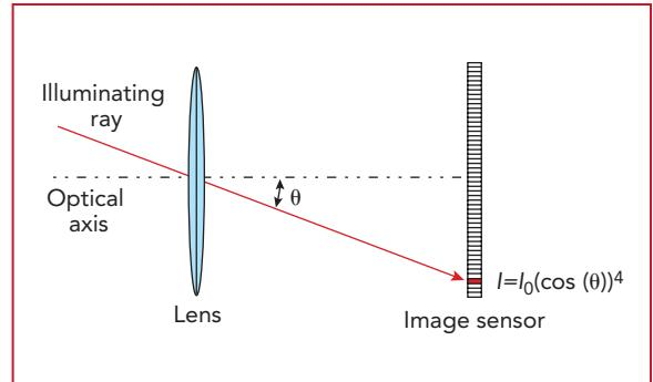
**FIGURE 5.** Image brightness naturally falls off toward a frame's edge.
