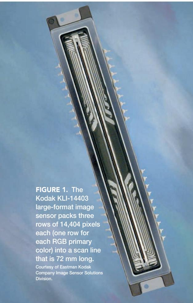
**FIGURE 1.** The Kodak KLI-14403 large-format image sensor packs three rows of 14,404 pixels each (one row for each RGB primary color) into a scan line that is 72 mm long.
