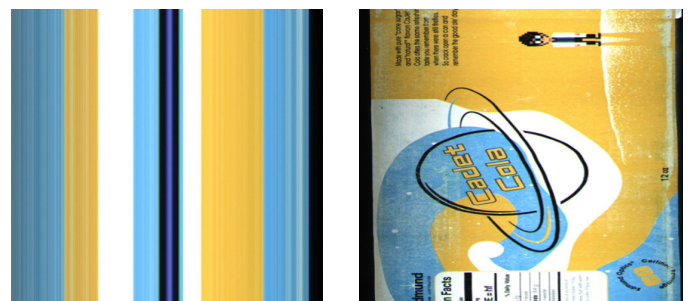
Figure 3 – A stationary object (left) and the same object in motion (right) captured with a line scan sensor
