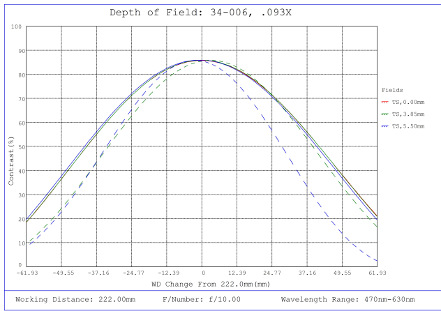
#34-006, 0.093X, 2/3" C-Mount TitanTL® Telecentric Lens, Depth of Field Plot, 222mm Working Distance, f10
