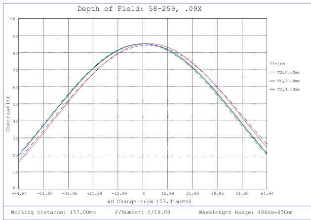
#58-259, 0.09X 1/2" GoldTL™ Telecentric Lens, Depth of Field Plot, 157mm Working Distance, f10
