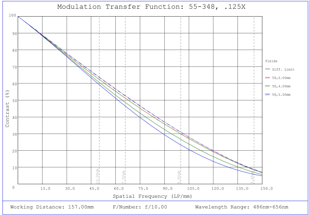
#55-348, 0.125X, 2/3" GoldTL™ Telecentric Lens, Modulated Transfer Function (MTF) Plot, 157mm Working Distance, f10
