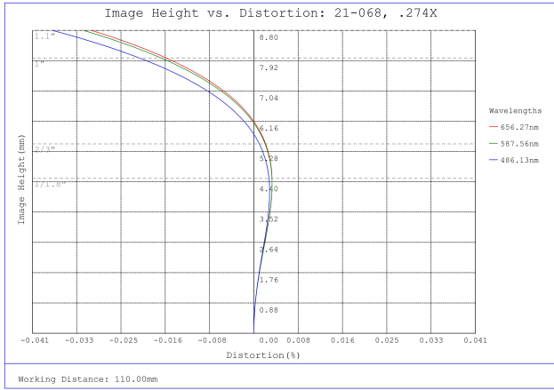
#21-068, 0.274X CobaltTL Telecentric Lens, Distortion Plot
