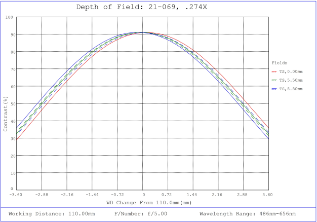
#21-069, 0.274X In-Line CobaltTL Telecentric Lens, Depth of Field Plot, 110mm Working Distance, f5
