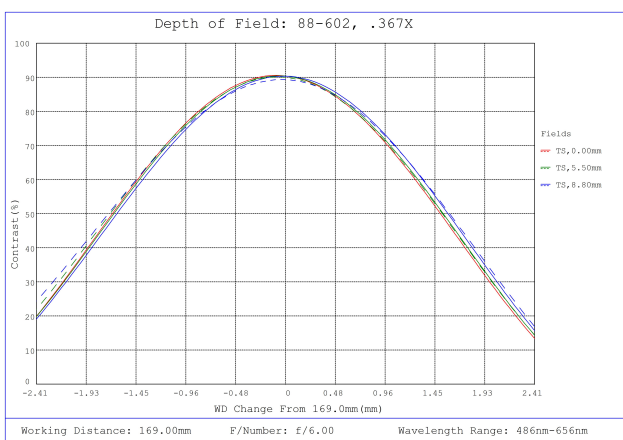
#88-602, 0.367X CobaltTL Telecentric Lens, Depth of Field Plot, 169mm Working Distance, f6
