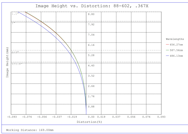
#88-602, 0.367X CobaltTL Telecentric Lens, Distortion Plot
