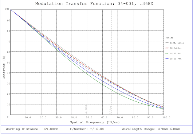
#34-031, 0.368X, 35mm F-Mount TitanTL® Telecentric Lens, Modulated Transfer Function (MTF) Plot, 169mm Working Distance, f16
