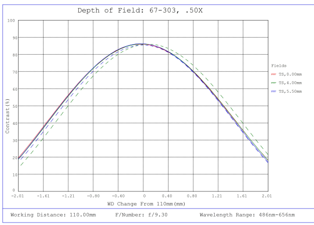
#67-303, 0.5X, 110mm WD, In-Line CompactTL™ Telecentric Lens, Depth of Field Plot, 110mm Working Distance, f9.3
