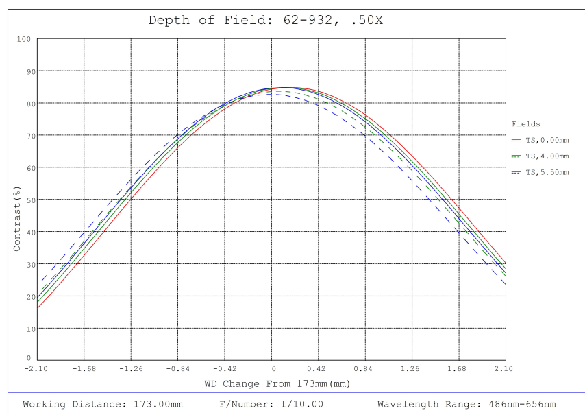
#62-932, 0.5X, 2/3" C-Mount PlatinumTL™ Telecentric Lens, Depth of Field Plot, 173mm Working Distance, f10
