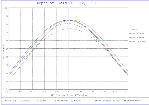
#62-912, 0.5X, 28.7mm F-Mount PlatinumTL™ Telecentric Lens, Depth of Field Plot, 175mm Working Distance, f10
