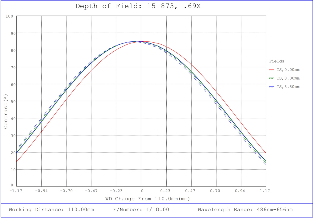
#15-873, 0.69X In-Line Illumination CobaltTL Telecentric Lens, Depth of Field Plot, 110mm Working Distance, f10
