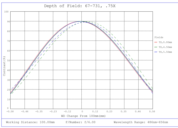
#67-731, 0.75X SilverTL™ Telecentric Lens, Depth of Field Plot, 100mm Working Distance, f6
