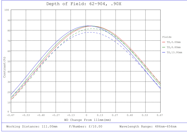
#62-904, 0.9X, 28.7mm M42 x 1.0 (19.53mm) PlatinumTL™ Telecentric Lens, Depth of Field Plot, 111mm Working Distance, f10
