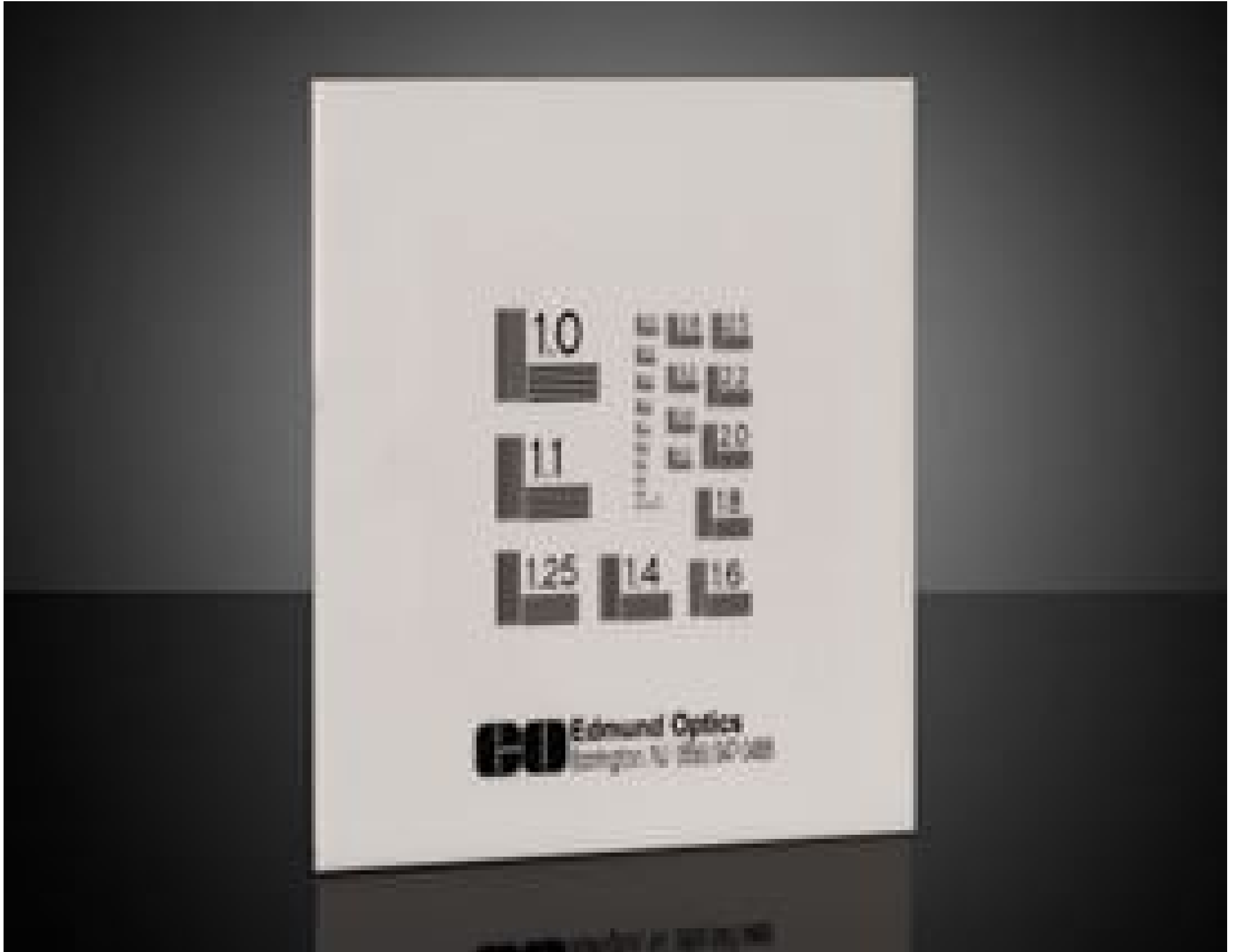
NBS 1963A Resolution Target
