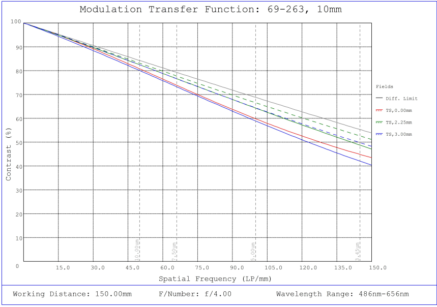
#69-263, 10mm FL f/4, Blue Series M12 Lens, Modulated Transfer Function (MTF) Plot, 150mm Working Distance, f4
