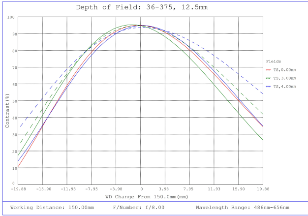
#36-375, 12.5mm FL f/8, Rugged Blue Series M12 Lens, Depth of Field Plot, 150mm Working Distance, f8
