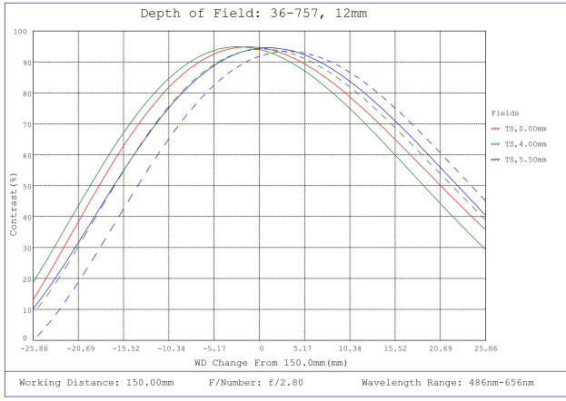
#36-757, 12mm f/2.8, 150-500mm Primary WD, HRi Series Fixed Focal Length Lens, Depth of Field Plot, 150mm Working Distance, f2.8
