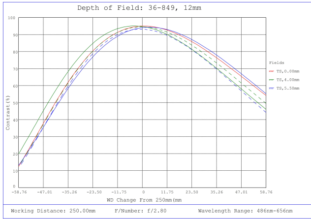
#36-849, 12mm f/2.8, 150-500mm Primary WD, HRr Series Fixed Focal Length Lens, Depth of Field Plot, 250mm Working Distance, f2.8
