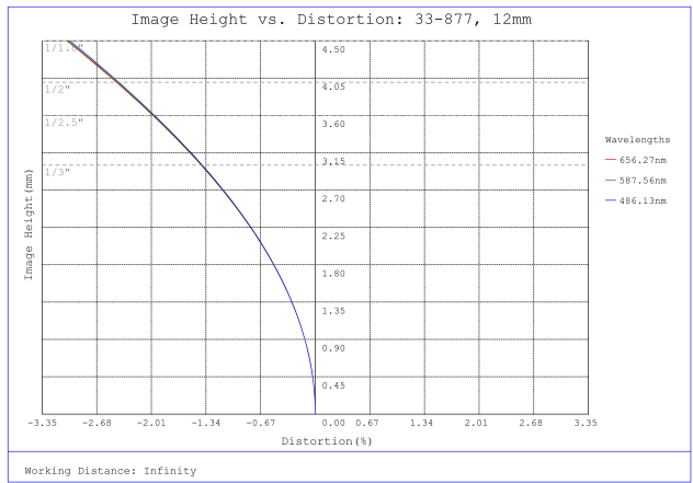
#33-877, 12mm, f/2.8 UCi Series Fixed Focal Length Lens, Distortion Plot
