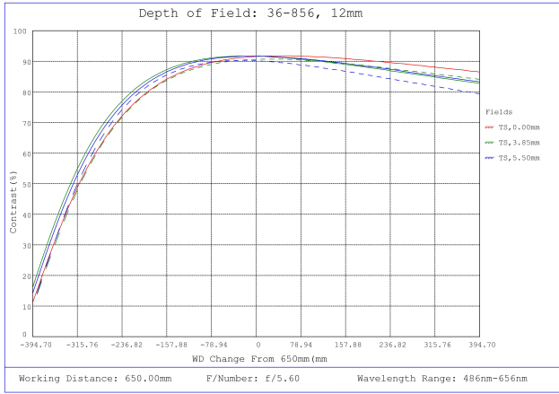
#36-856, 12mm f/5.6, 400-2000mm Primary WD, HRr Series Fixed Focal Length Lens, Depth of Field Plot, 650mm Working Distance, f5.6
