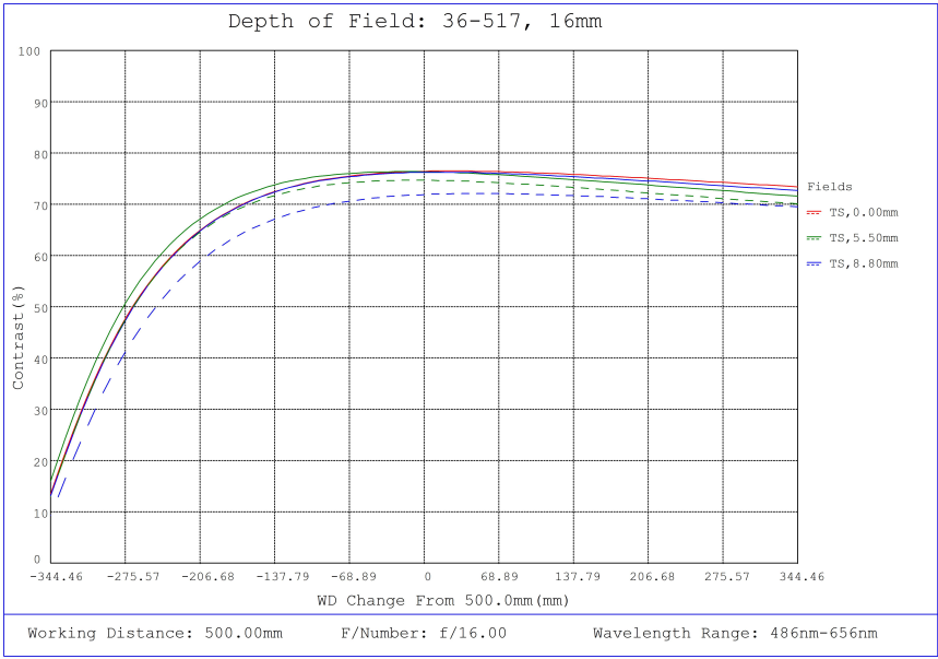
#36-517, 16mm f/16, HPr Series Fixed Focal Length Lens, Depth of Field Plot, 500mm Working Distance, f16
