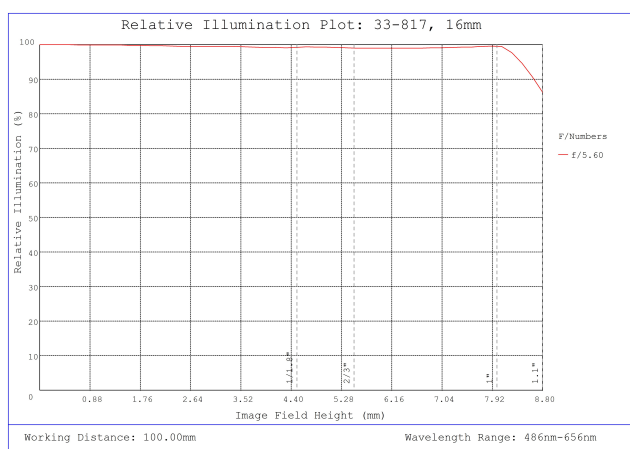
#33-817, 16mm f/5.6, HPI Series Fixed Focal Length Lens, Relative Illumination Plot
