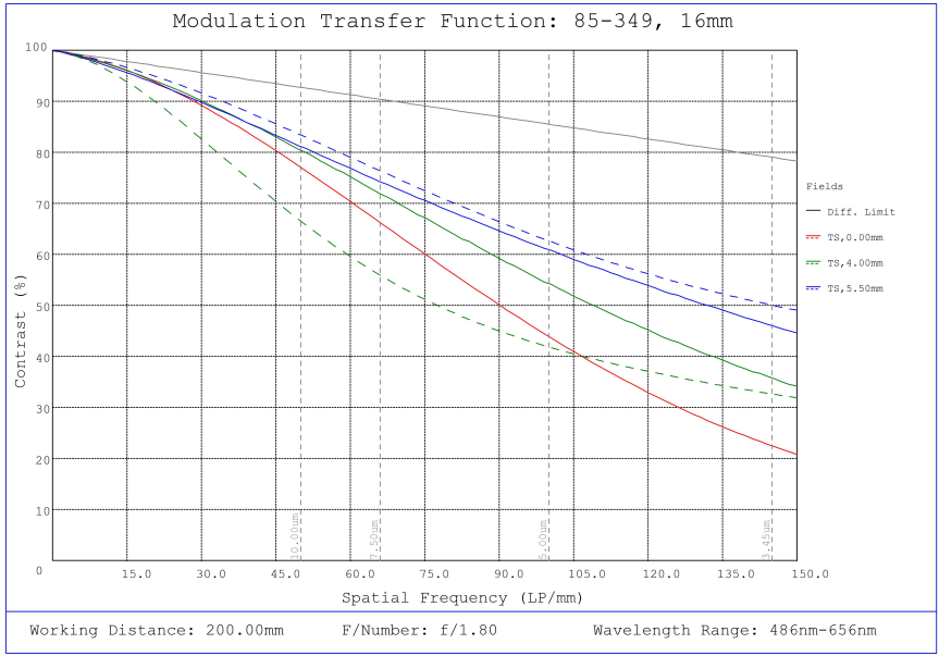
#85-349, 16mm, f/1.8 Ci Series Fixed Focal Length Lens, Modulated Transfer Function (MTF) Plot, 200mm Working Distance, f1.8
