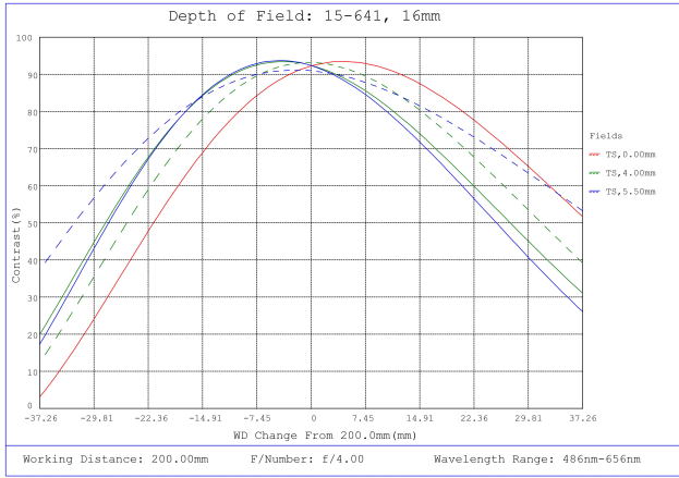
#15-641, 16mm, f/4 Cw Series Fixed Focal Length Lens, Depth of Field Plot, 200mm Working Distance, f4
