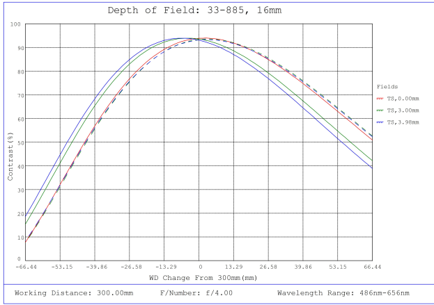
#33-885, 16mm, f/4 UCI Series Fixed Focal Length Lens, Depth of Field Plot, 300mm Working Distance, f4
