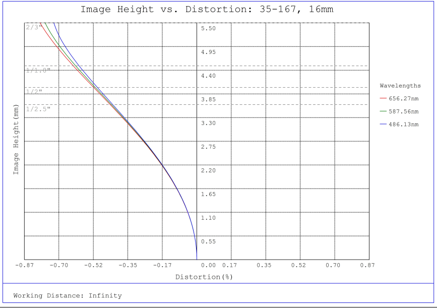
#35-167, 16mm, f/5.6 Cr Series Fixed Focal Length Lens, Distortion Plot
