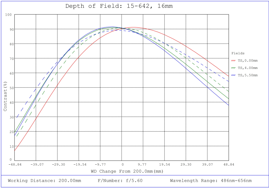
#15-642, 16mm, f/5.6 Cw Series Fixed Focal Length Lens, Depth of Field Plot, 200mm Working Distance, f5.6
