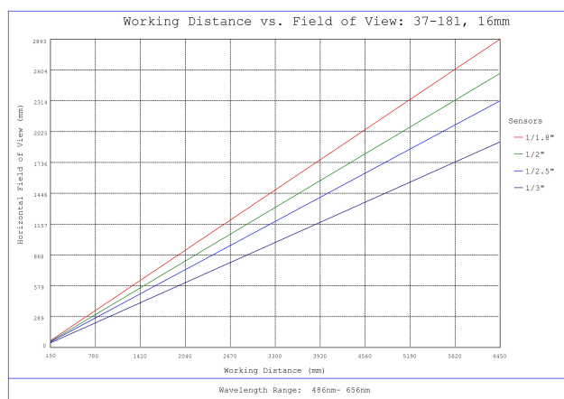
#37-181, 16mm FL f/2.5 Blue Series M12 Lens, Working Distance versus Field of View Plot
