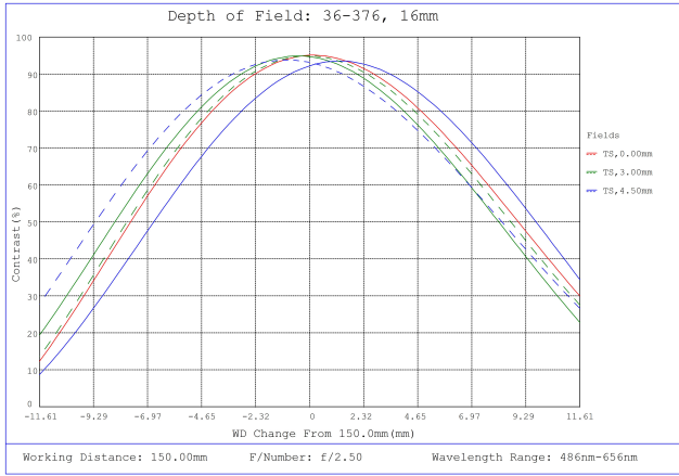
#36-376, 16mm FL f/2.5 Rugged Blue Series M12 Lens, Depth of Field Plot, 150mm Working Distance, f2.5
