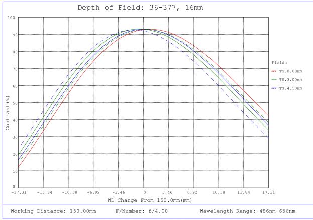
#36-377, 16mm FL f/4.0 Rugged Blue Series M12 Lens, Depth of Field Plot, 150mm Working Distance, f4
