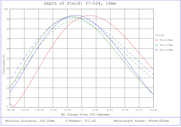
#37-524, 16mm FL, Liquid Lens M12 Lens, Depth of Field Plot, 200mm Working Distance, f2.4
