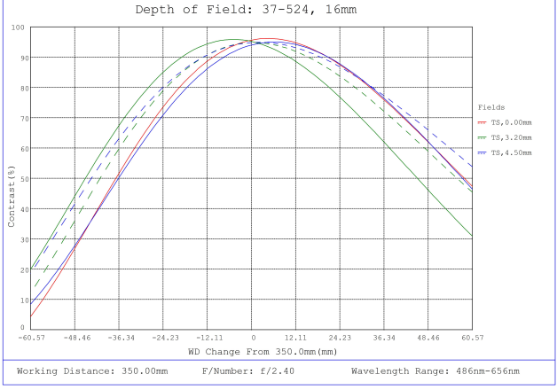
#37-524, 16mm FL, Liquid Lens M12 Lens, Depth of Field Plot, 350mm Working Distance, f2.4
