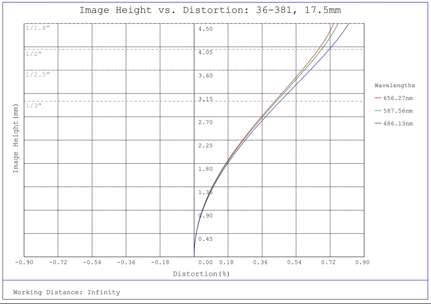
#36-381, 17.5mm FL f/4, Rugged Blue Series M12 Lens, Distortion Plot
