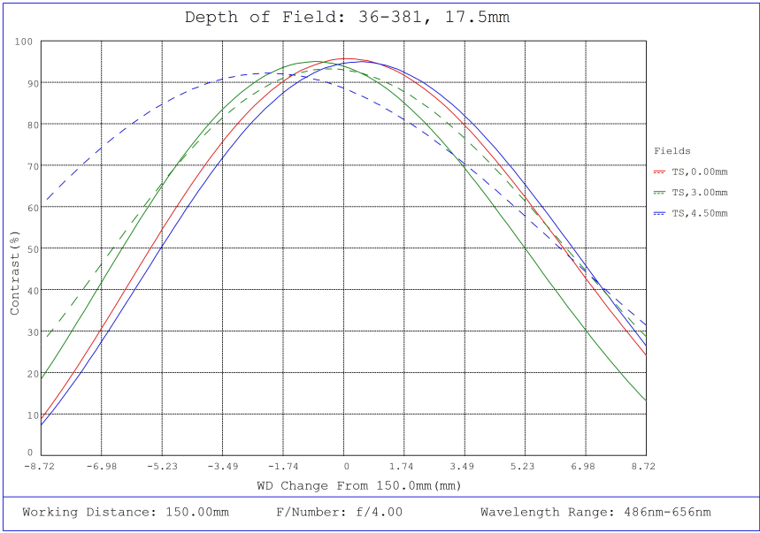
#36-381, 17.5mm FL f/4, Rugged Blue Series M12 Lens, Depth of Field Plot, 150mm Working Distance, f4
