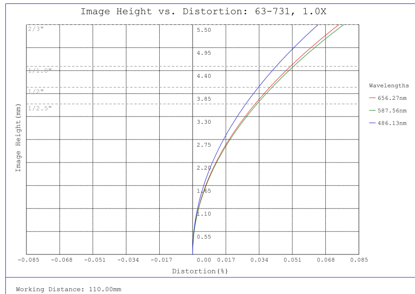
#63-731, 1X, 110mm WD CompactTL™ Telecentric Lens, Distortion Plot
