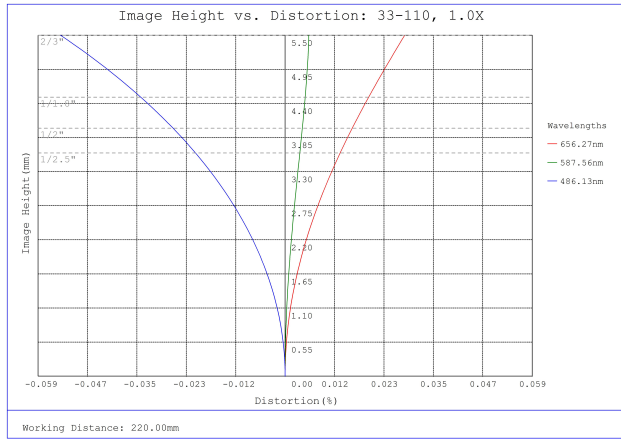
#33-110, 1X, 220mm WD, In-Line CompactTL™ Telecentric Lens, Distortion Plot
